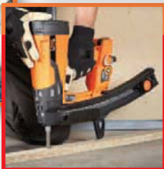
● Wood plank fixing onto concrete
