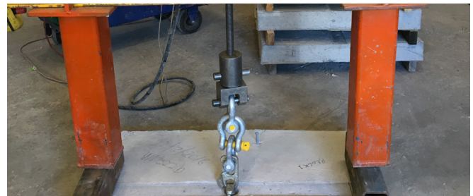
Figure 4: 1FA045 Foot Anchor tested in tension.
