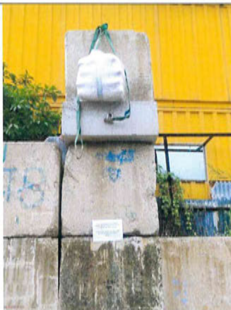
Set up of dead weight for 2.0m drop height
