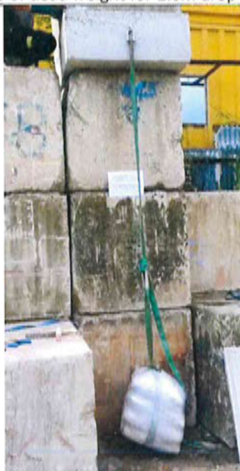
Free release of dead weight for 2.0m drop height
